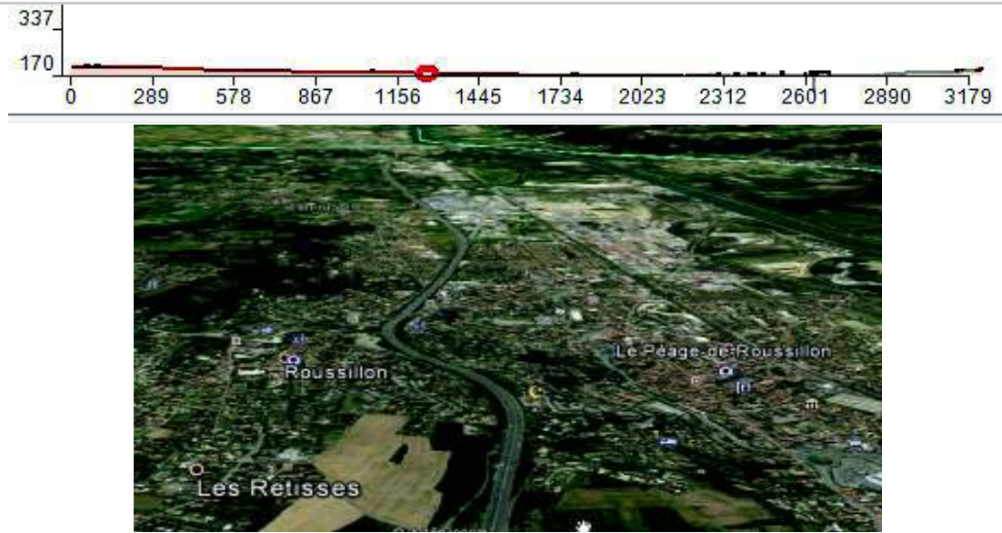
Illustration 41: A7 St-Rambert d'Albon – Tain l'Hermitage. Typical cross-profile on this section. Red dots mark the location of road infrastructure modelled as acoustic sources. Horizontal and vertical scales in meters and aerial view (GoogleEarth) close to Roussillon.
