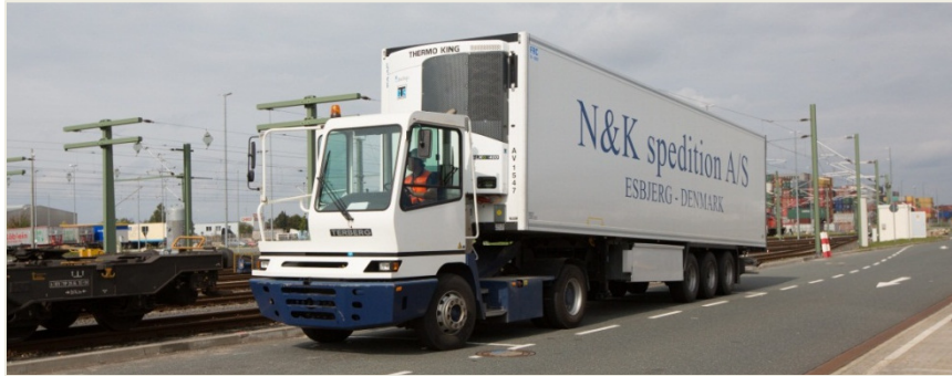
Figure 25: Terminal tractor with coupled semitrailer 108
