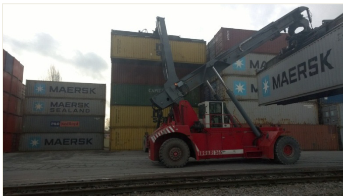
Figure 24: Transshipment of container with reach stacker 106
