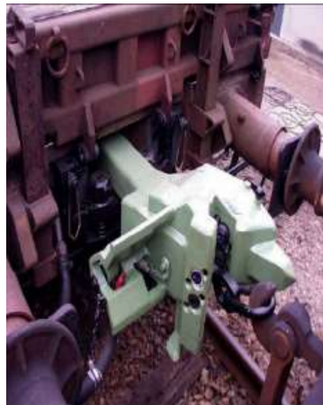
Photo 10: Coupling with conventional screw-coupler
