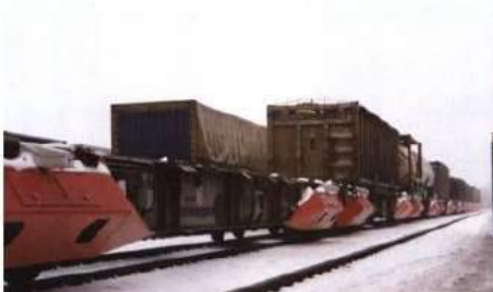
Photo 3: Bogie skirts for noise protection
