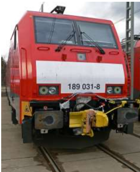
Photo 9 Locomotive with C-AKv coupler
