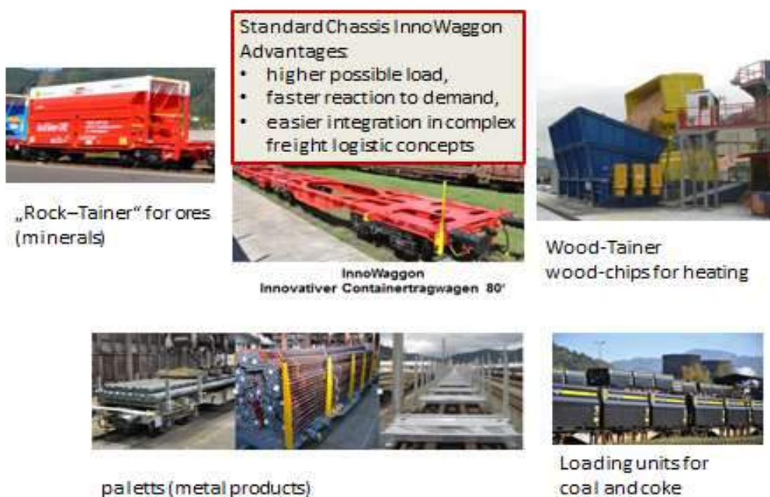
Figure 4: Separation of chassis and loading unit, example Rail Cargo Group Austria
