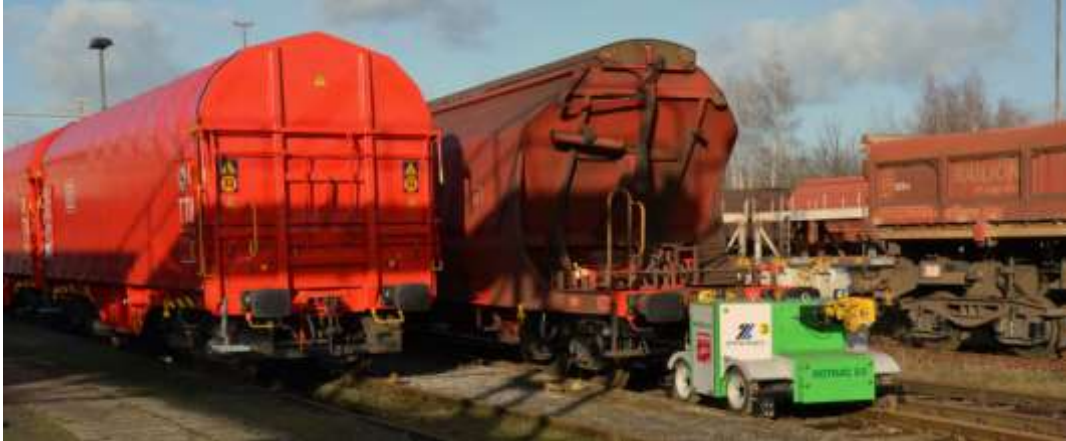
Photo 11: Small automatic two-way shunting robot in the wagon repair shop in Paderborn
